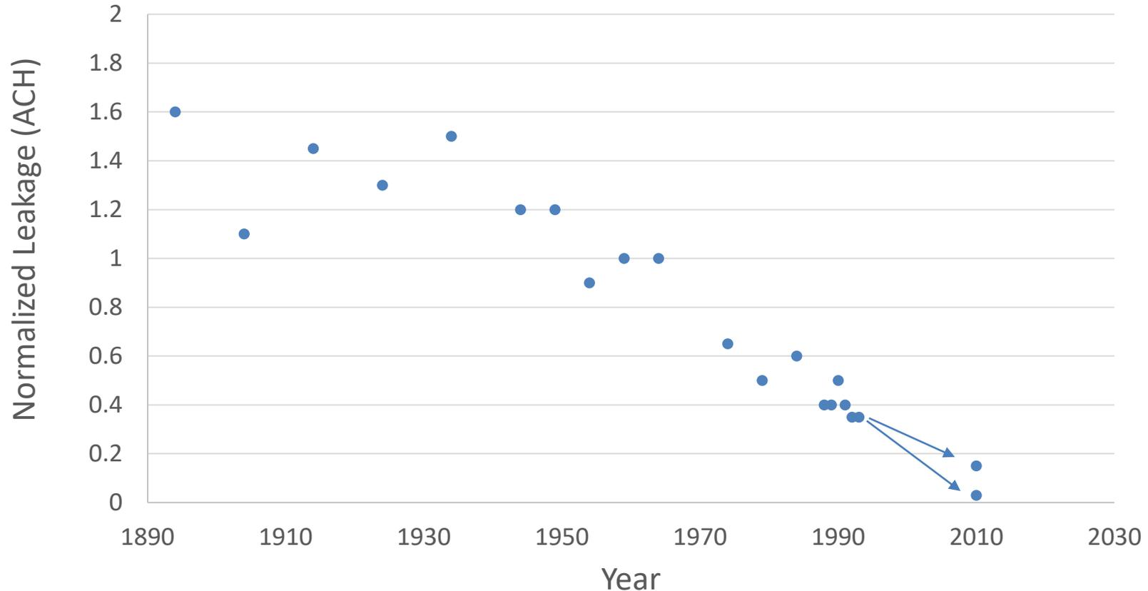
2010 data represents good construction (3ACH at 50Pa) and “Passive House” construction (0.6ACH at 50Pa)
