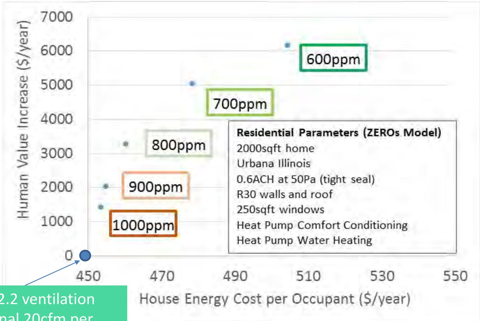
ASHRAE 62.2 ventilation with nominal 20cfm per person of ventilation results in ~1100ppm CO2
