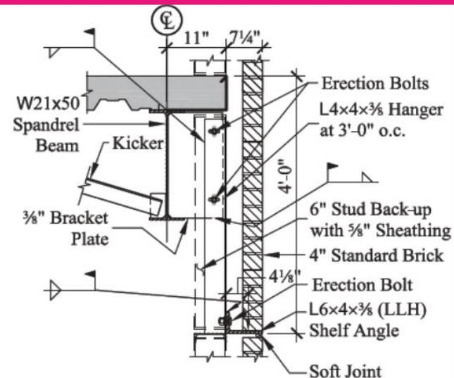
Fig. 7-17. Section of spandrel beam with hanger system.
