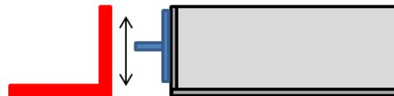
*Additional plate with stud pre-welded can be field-adjusted on slab
