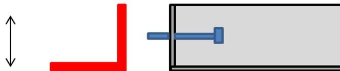
*Angle height is adjustable due to long slotted holes*
