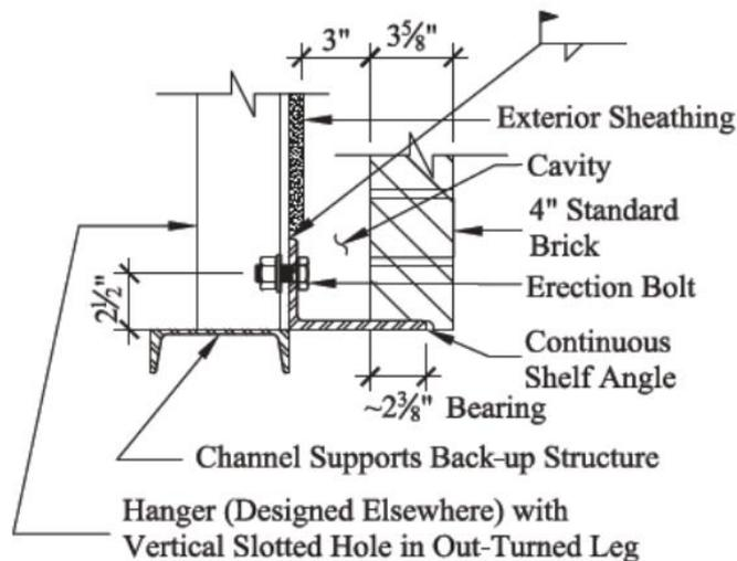
Fig. 7-16. Section of shelf angle supporting brick veneer.
